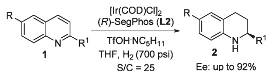
Scheme 13. Asymmetric Hydrogenation of Quinolines 1 Activated with Brønsted Acid
